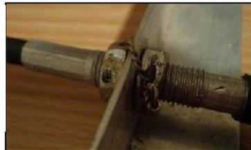
This method pictured shows the nuts being drilled and locks wired. Nuts are locked and cannot come undone. (Righty tightly, lefty loosely)
