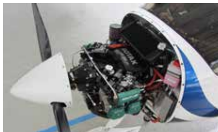
The Rotax 912 iS fuel injected engine is neatly fitted and provides easy working space
