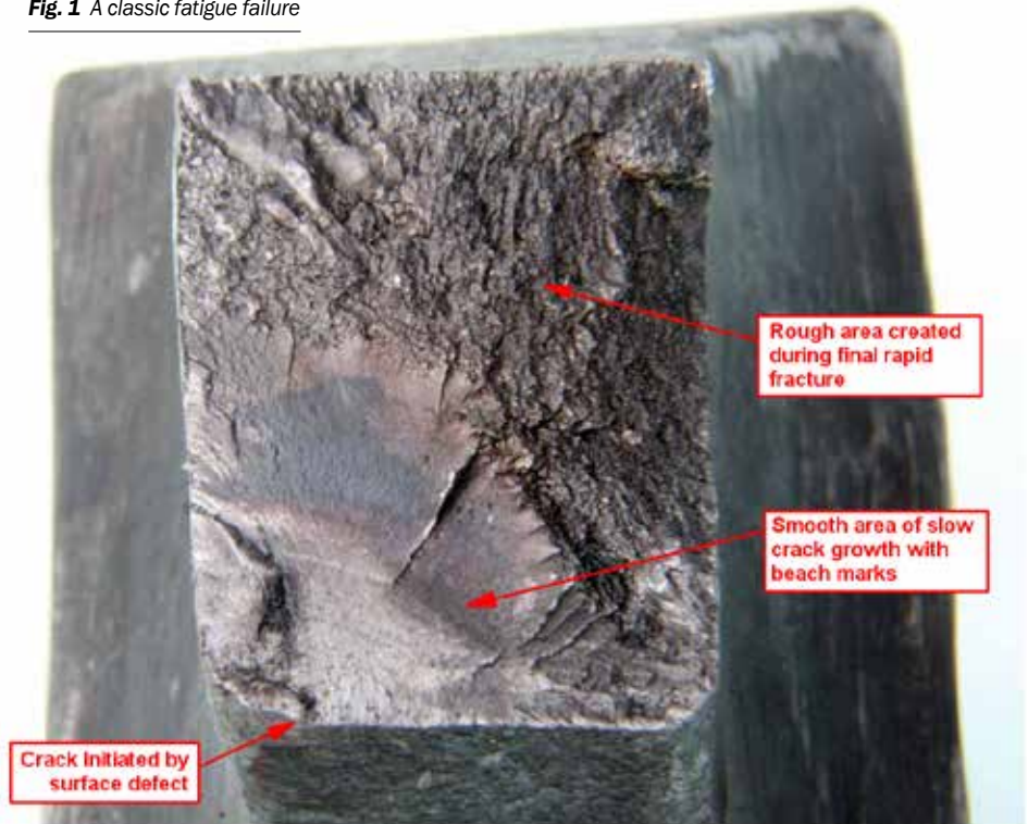
Fig. 1 A classic fatigue failure
