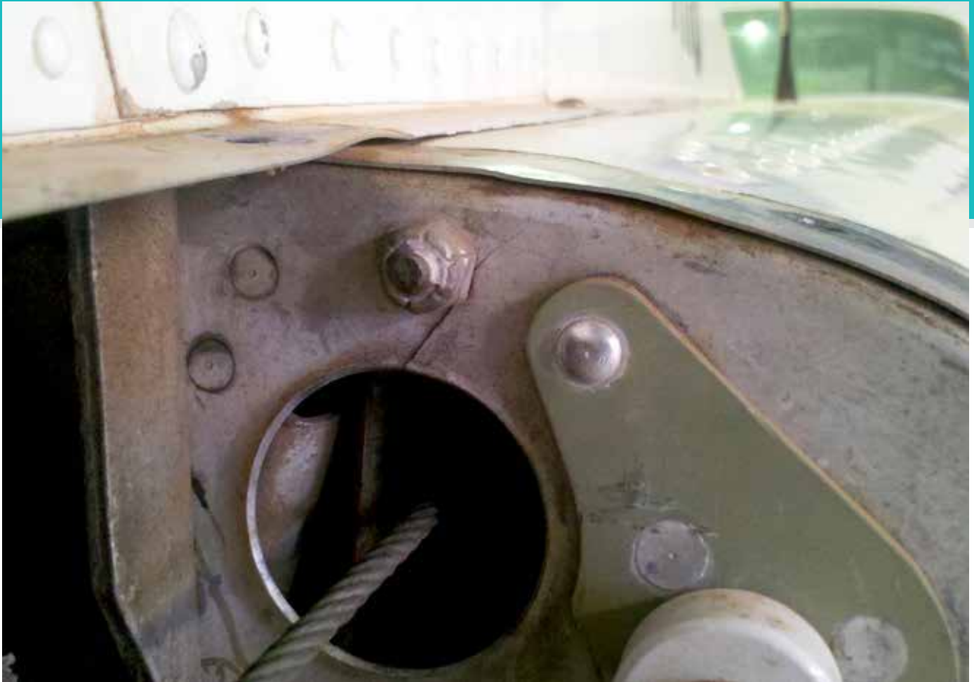
Fig. 2 (above) Fatigue cracks frequently initiate at holes.
