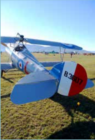
Bruce Clarke's latest project, a full scale replica Nieuport 17 at the Brisbane Valley air show. Powered by a 2275cc VW engine. The original plans were by Graham Lee from Canada. Photo: Alan Betteridge
